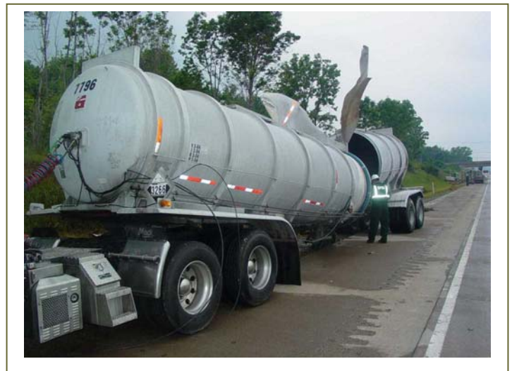
Bulk chemicals greatly increase the possibility of a major incident. This tanker was shipping bulk chlorinated CIP cleaner
